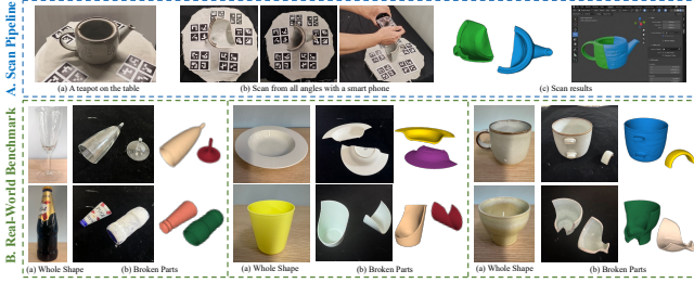
Fig. 3. Part A illustrates the pipeline for scanning and reconstructing real objects. Part B presents examples of fractured parts from various categories.
